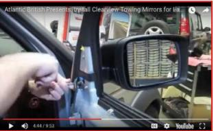
**9.** Run out the three bolts holding the mirror in place, taking caution to support the mirror, so not to drop it.
