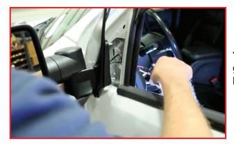
**18.** Hand-tighten the nuts to the three bolts to hold the mirror. Secure the bolts with a rachet, applying a few turns to each in a equal pattern.
