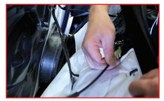
**9.** Disconnect the door handle connection wire, and take the time to detach the other 3 connecting wires. The wires have safety releases. Take a small flathead screwdriver and pull down the red tab, and the connections will pinch and pull out.
