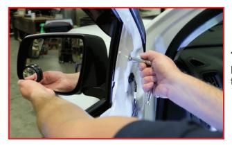
**13.** Run out the three bolts holding the mirror in place, taking caution to support the mirror, so not to drop it.
