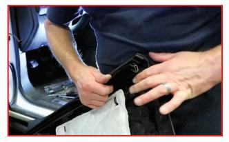
**21.** Reinstall the door panel. Start by sliding the weatherstripping off the top of the door panel. Remove the 5 clips across the top and insert into 5 slots of the door frame. Clip weatherstrip on, fuzzy side towards the window glass.
