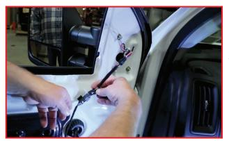
**19.** Plug in the connector that pertains to your vehicle model. The mirror is now installed. Test the mirror for operation. There will be an extra connector that you will <u>NOT</u> use — just tuck it away when replacing the door panel.
