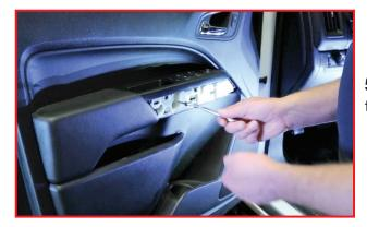
**5.** Once the screws are fully loosened, use a magnet to retrieve them from the door panel recess.
