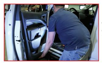
**7.** With the five screws removed, pop off the door panel, starting at the bottom, using trim removal tool, releasing the pop pins.
