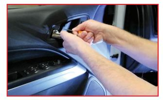
**1.** First the door panel must be removed to access the side mirror connector: Using a pocket screwdriver or pick tool, pry the cover as shown from behind the door handle.
