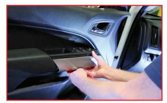
**3.** Remove the trim on the door panel arm rest using a plastic trim panel removal tool.
