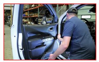
**23.** Mount the door panel by hand and engage pin clips. Start from the top, by slipping door panel over door lock, and work your way around panel, pushing on the door panel where the pop pins insert, until the pin clips engage.
