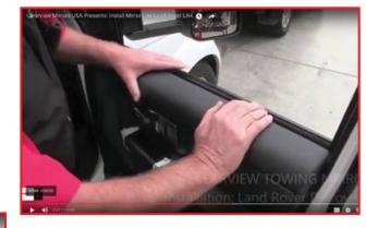
23. Re-install the 2 screws at the bottom of the door panel.
