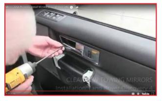
**25.** Re-install the one screw behind the door handle.
