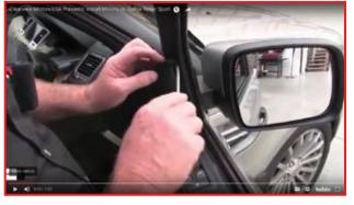
**1.** First the trim cover for the side mirror must be removed to access the side mirror connector. Use a pocket screwdriver to pry loose.
