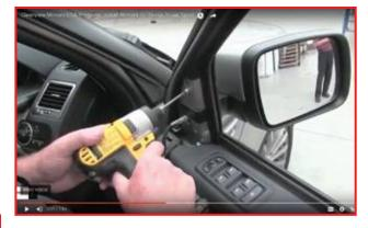
7. Remove the original side mirror by snaking wiring through opening.
